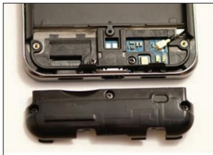
▲ Fig. 2 Antenna integrated into the package.<sup>2</sup>
