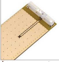
▲ Fig. 3 Discrete antenna mounted to a PWB.<sup>3</sup>
