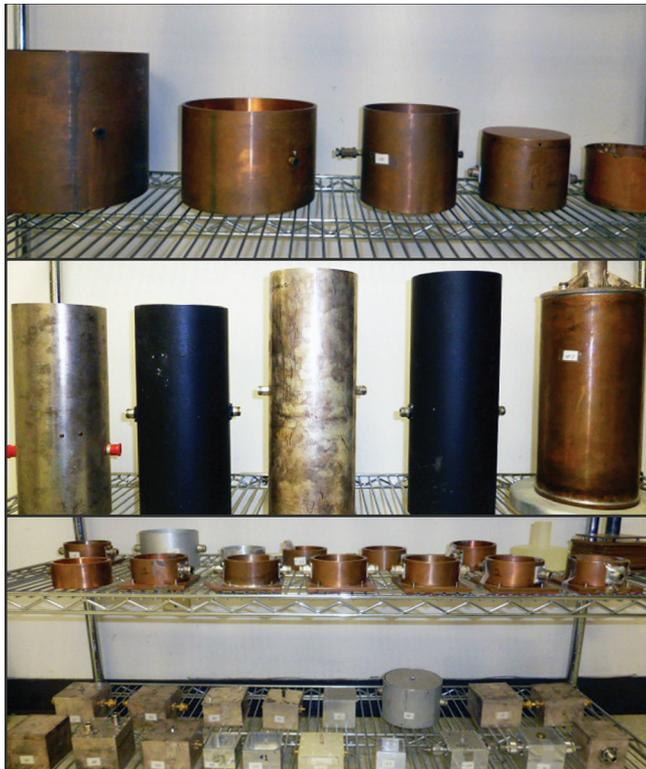
▲ Fig. 7 Custom resonator test cavities.
